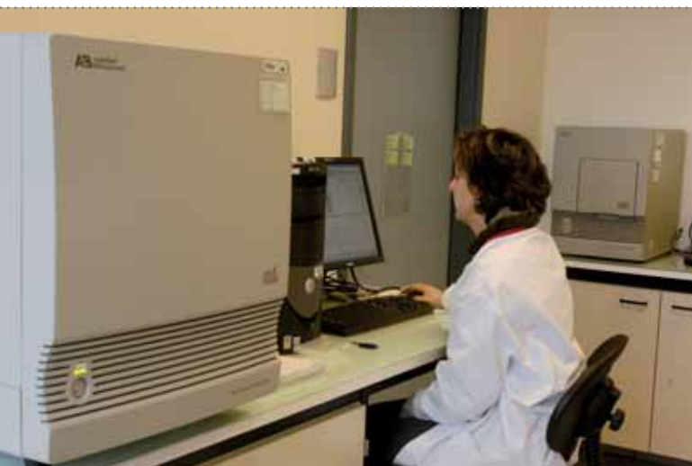
DNA Vision is equipped with ABI SDS for low or high throughput SybrGreen / TaqMan / TLDA assays
